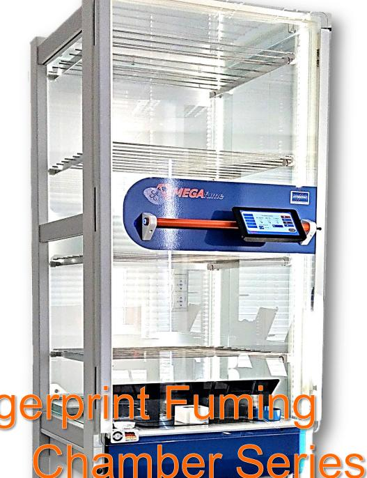
for the development of fingerprints on non-porous surfaces using fluorescent & non-fluorescent cyanoacrylates in liquid and powder form
